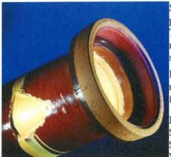
Sewer Lateral and Main LineSectional Lining System is a cured-inplace sectional system for the repair of damaged sewer pipelines. The patch is a composite of two basic materials - a fiberglass matting impregnated with an ambient curing two-part silicate resin system.
