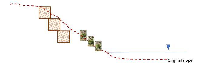
Excavate bank, place blocks. Lowest row of blocks is buried and serves as a foundation. Upper two rows of blocks could serve as public seating/viewing. Plant with bankside vegetation that would inhibit foot traffic (speckled alder, red osier dogwood).
