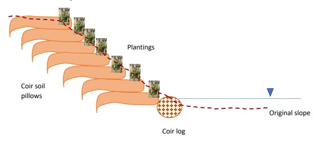
Excavate back slope, stake coir log along water's edge, lay down fine mesh coir blanket, cover blanket with 12-18 in. of excavated material, then wrap fill with blanket, staking blanket ends together on landward side. Continue adding soil pillows in stepwise fashion to match existing slope up to elevation of existing path. Plant soil pillows with bankside vegetation that would inhibit foot traffic (speckled alder, red osier dogwood). Another view of system is below.
