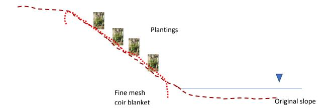
Excavate key trenches at upper and lower extent of coir blanket, scarify slope, broadcast seed mixes (wildflower, sedges, grasses, forbs) rake in seeds, lightly compact, cover with coir blanket, fill key trenches, stake blanket with wooden stakes, plant live stake or bushes.
