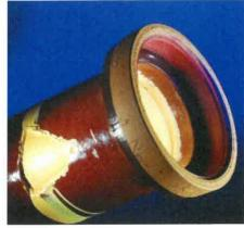
Sewer Lateral and Main LineSectional Lining System is a cured-inplace sectional system for the repair of damaged sewer pipelines. The patch is a composite of two basic materials - a fiberglass matting impregnated with an ambient curing two-part silicate resin system.
