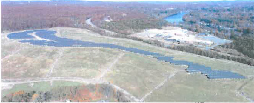
This aerial view shows the large solar array built on Manchester's capped landfill, turning seemingly unusable land into a benefit. Photo Provided by Kearsarge Energy
