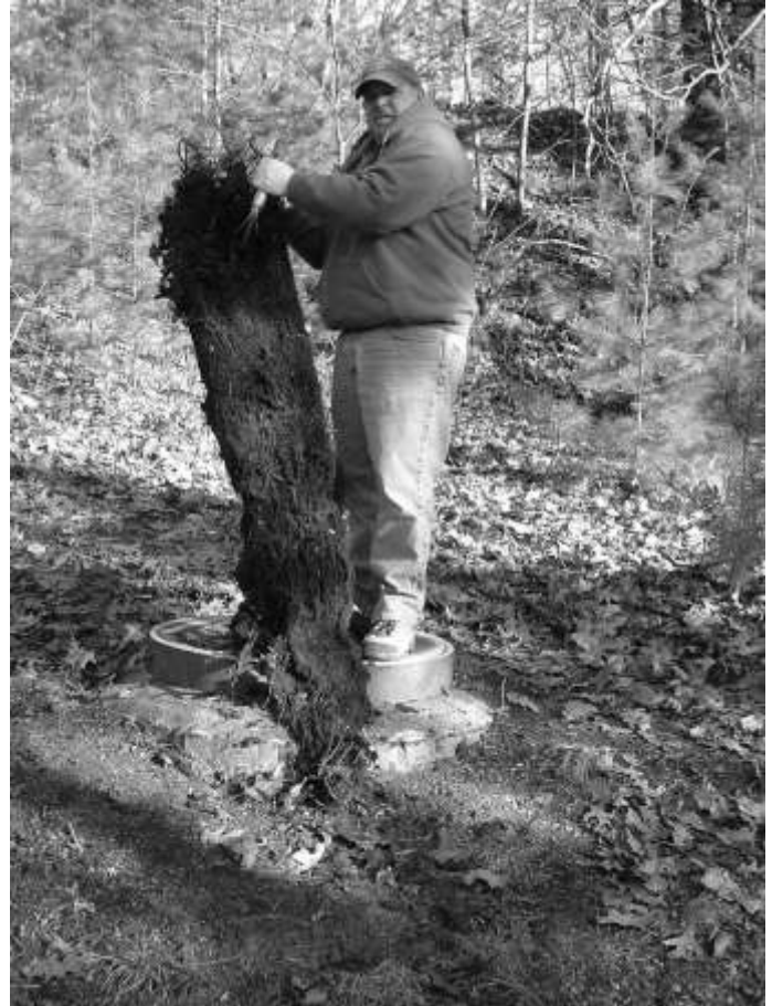
ABOVE: The largest of several roots removed from the effluent discharge pipe.
